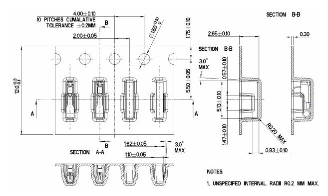
The Universal Contact has a very low mass and due to this it can not be guaranteed that the component will sit fully flat in the base of the pocket when viewed in the tape. However, during the feeding and indexing of the machine, the natural vibration should settle the component down into the pocket. Should the vibration not re-position the contact fully the use of the correct nozzles and settings during pick and place will rectify this situation.
