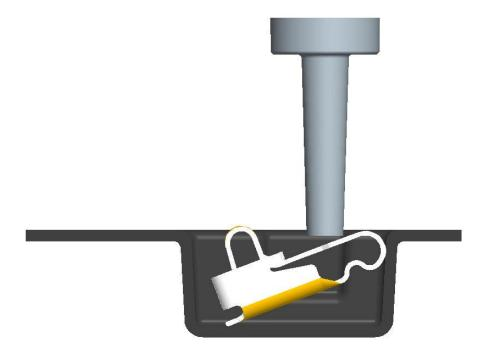
Once the cover tape is removed from the pocket, if the vibration and shock of the feeding mechanism on the machine is too violent, the contacts could jump out of position in the tape, or even jump out of the pocket due to their low mass.
