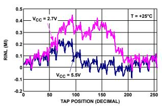
FIGURE 12. RINL vs TAP POSITION IN RHEOSTAT MODE FOR 50k $\Omega$  (U)
