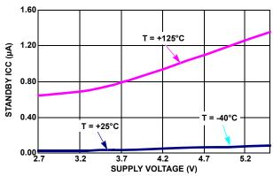
FIGURE 2. STANDBY ICC vs VCC
