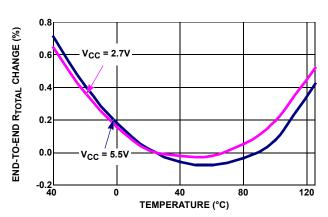
FIGURE 15. END-TO-END R<sub>TOTAL</sub> % CHANGE vs TEMPERATURE, 10k (W)
