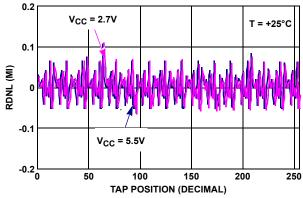
FIGURE 11. RDNL vs TAP POSITION IN RHEOSTAT MODE FOR 50k $\Omega$  (U)
