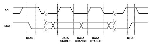
FIGURE 17. VALID DATA CHANGES, START, AND STOP CONDITIONS
