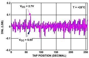
FIGURE 9. DNL vs TAP POSITION IN RHEOSTAT MODE FOR 50k $\Omega$  (U)
