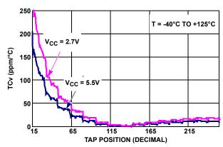
FIGURE 14. TCv FOR VOLTAGE DIVIDER MODE 10k (W) IN ppm
