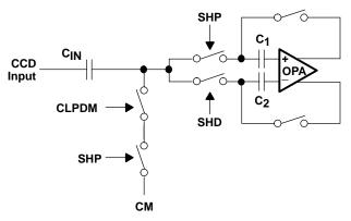
Figure 2. Block Diagram of CDS and Input Clamp
