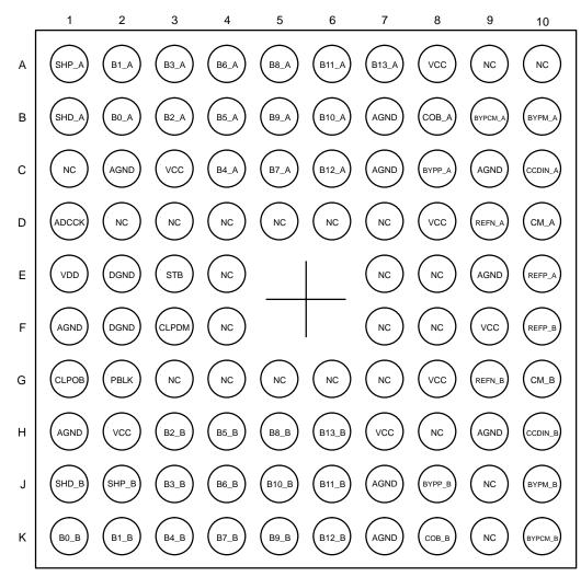
NOTE: The corner of the A1 position is indicated on the device top by a dot.
