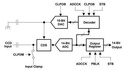
Figure 1. Simplified Block Diagram of VSP2254 (One Channel)
